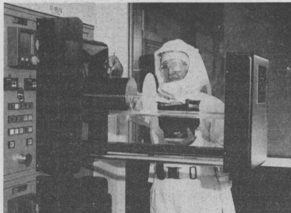
A TECHNICIAN working in the Microelectronics Development Lab loads silicon wafers into a furnace for heating integrated circuits. Sandia uses its world-class MDL facility for much of its cooperative research efforts with SEMATECH.
